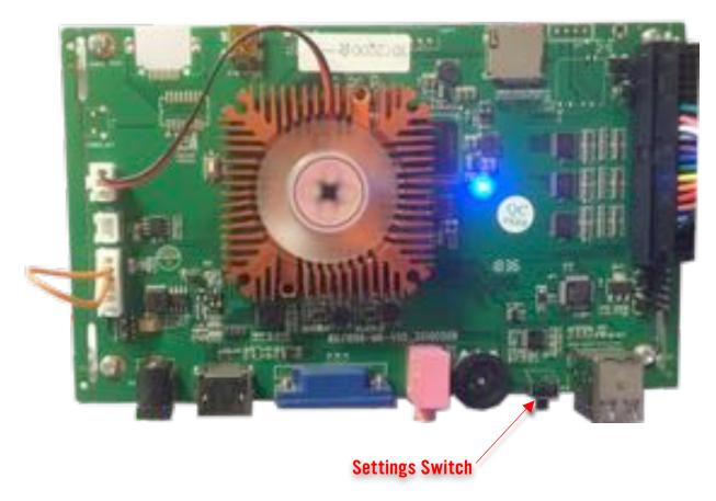
To access the options on your unit, open the access door using the machine's included key and locate the main circuit board inside. Press the small switch as illustrated.
